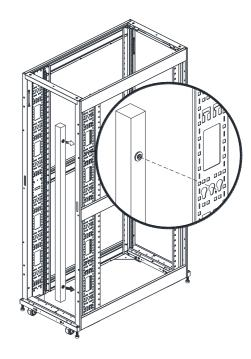
B: Mounting the Rack PDU on the PDU brackets of Al Ready Rack.
