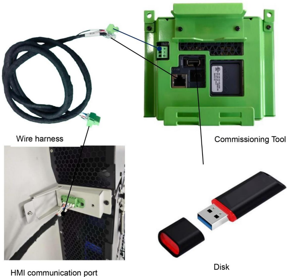
Figure 50. Commissioning Tool Connection
