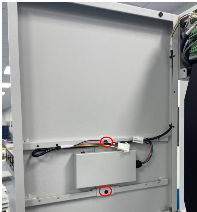
Figure 132. LED Light Module Removal
