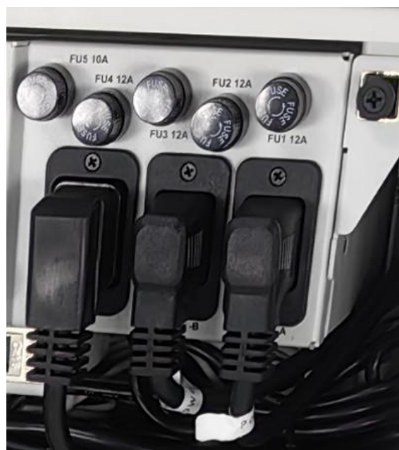
Figure 47. Power Cord Connection
