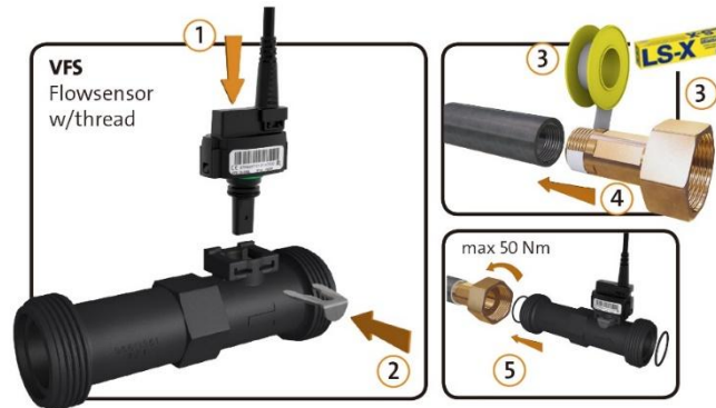
Figure 56. Installation Diagram
