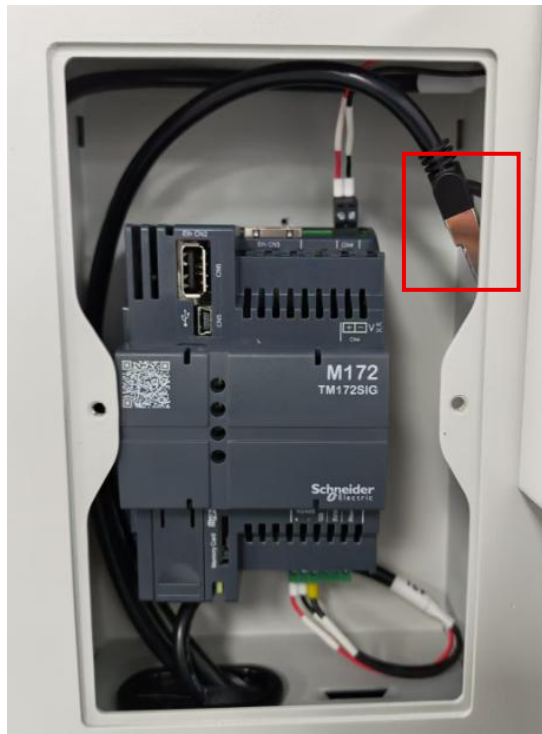
Figure 175. Unplug the connector from gat way module
