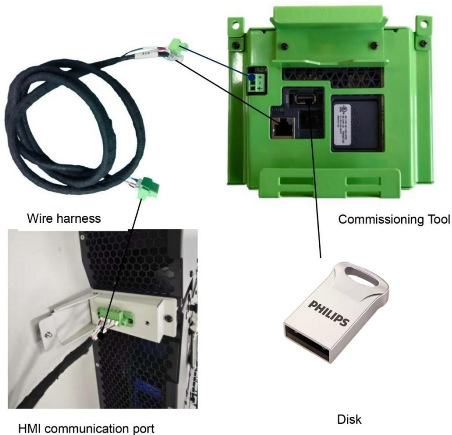
Figure 55. Commissioning Tool Connection
