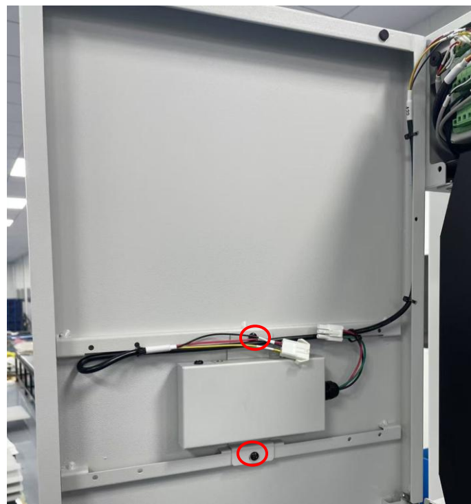
Figure 179. LED Light Module Removal
