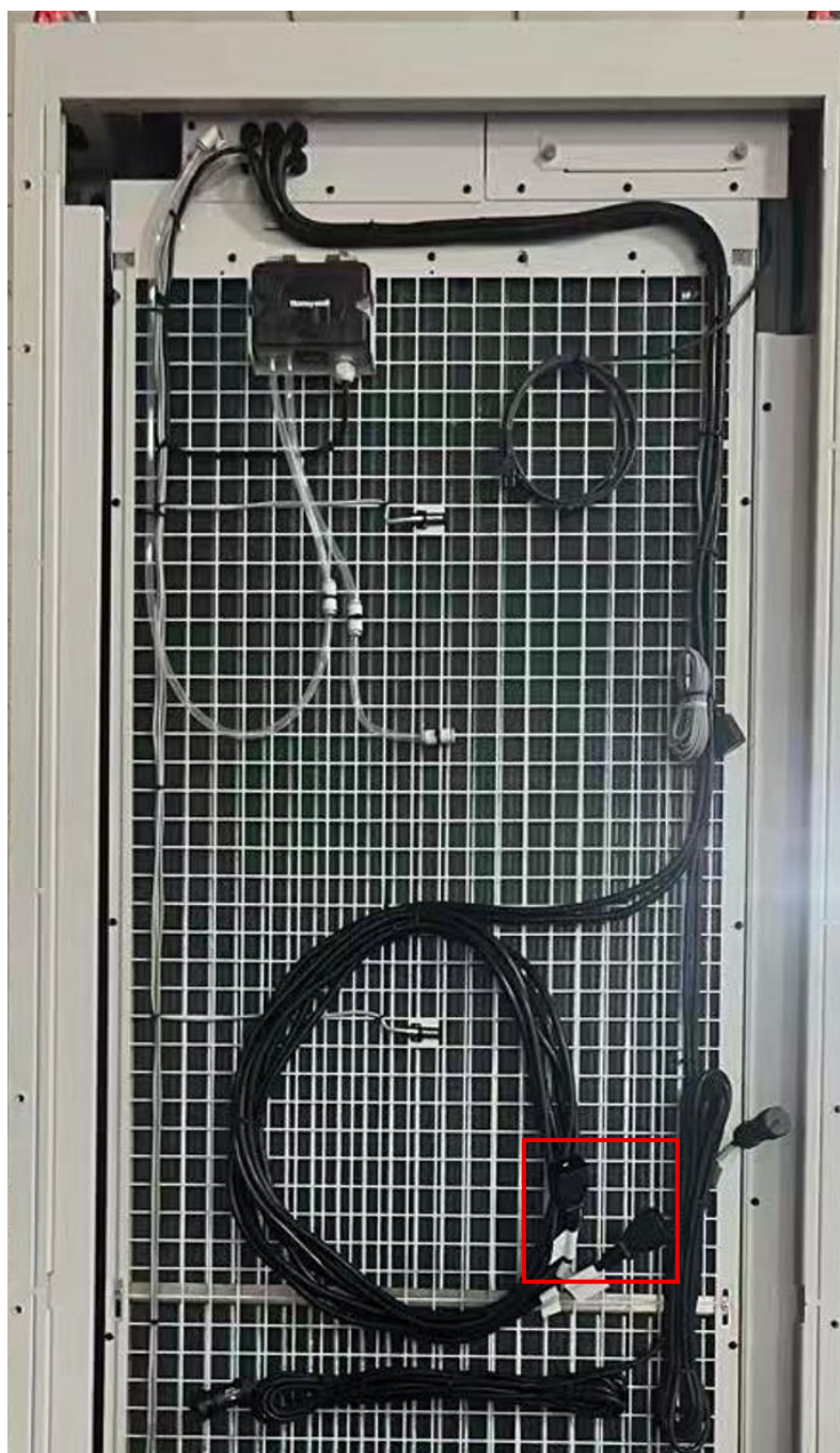
Figure 53. Connect power cords to the power supply
