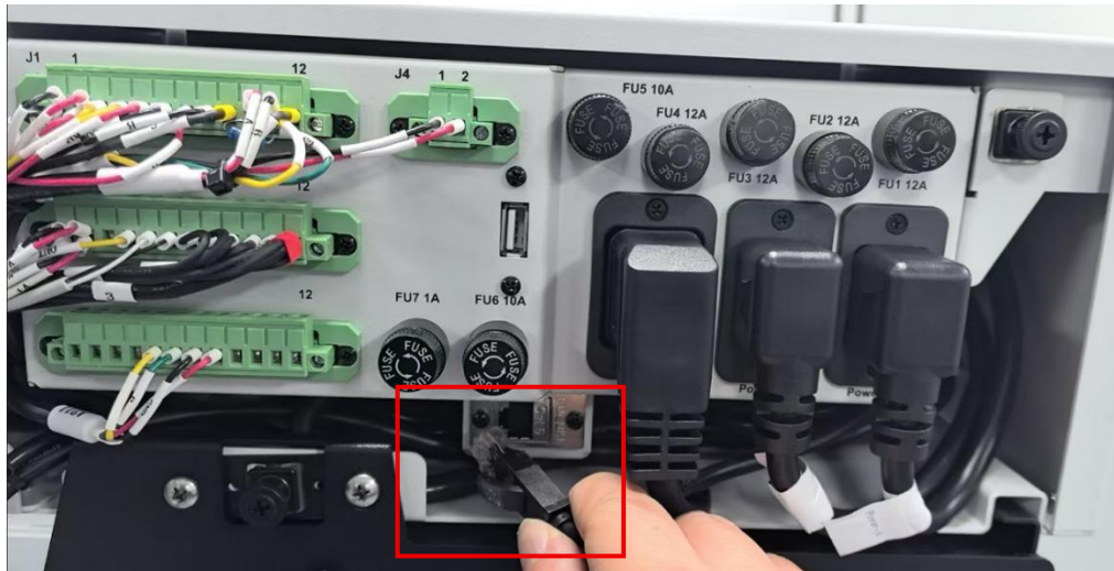
Figure 171. Unplug the network cable
